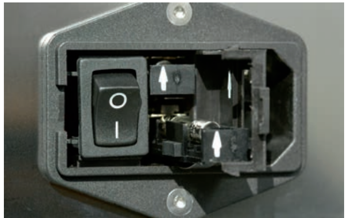
Figure 2.0: Opened fuse receptacles
