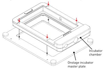
2. Attach the vessel holder/adaptor to the incubator chamber using the four thumb screws (indicated by red arrows).
