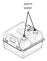
7. Place the water reservoir into the Control Unit with the fill holes to the front and close the lid.
